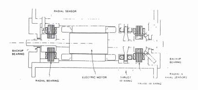
fields were properly adjusted, a two hundred fold reduction in midspan orbit at the first critical speed was achieved. The magnetic fields were also adjusted to minimize the vibration transmitted to the foundation. A two hundred fold reduction in the synchronous transmitted vibration was also achieved. We are about to begin a detailed testing program to supplement these results.
